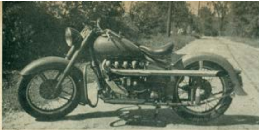
This model is one of the 1941 800 cc. experimental fours equipped with crash-bars and solo seat.
