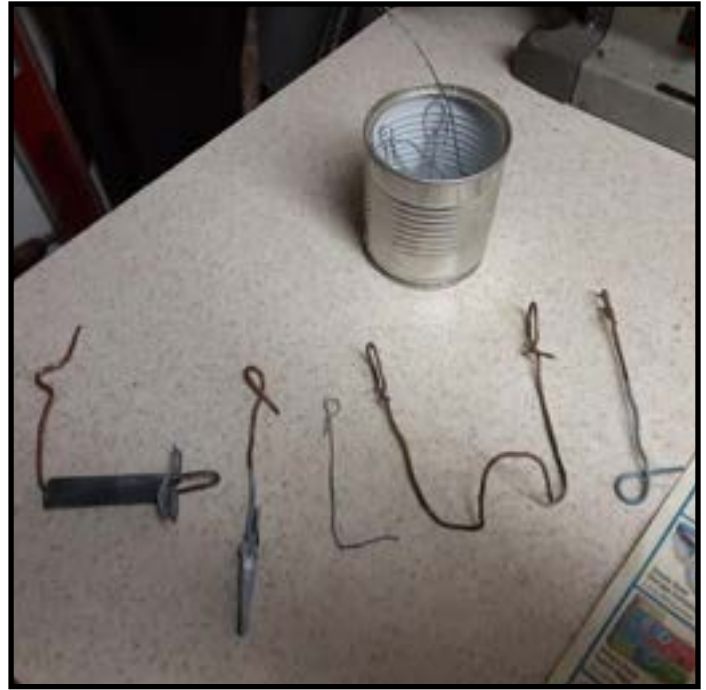
Here is an assortment of hangers to suspend parts from the top hanger wire. Note that they are nothing fancy. The thin wire is stainless safety wire. The heavy wire is 12 ga. house wiring. The small gray tube to the left was a set-up I made to plate the inside of a hollow part.
