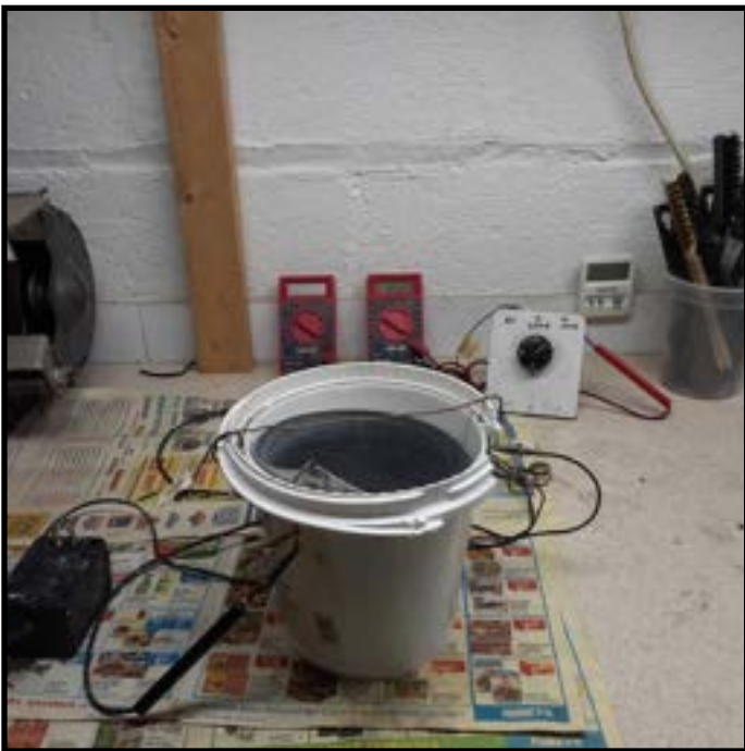
Here is my set-up. Starting at the left, the power supply. Plastic bucket, lined with zinc roofing sheeting, 2 Harbor Freight Multi-meters, an Ohmite potentiometer to control the power to the bath, a timer and a bucket of brushes.
