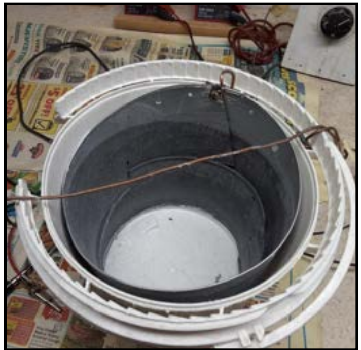
Here is the inside of the bucket. You can see the negative wire (hanger wire) running across the top and the positive wire connected with a screw to the zinc sheeting inside the bucket.
