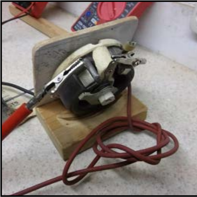
Here is the back side of the Ohmite potentiometer showing the electrical connection. Also gives you an idea of what you are looking for in a potentiometer.
