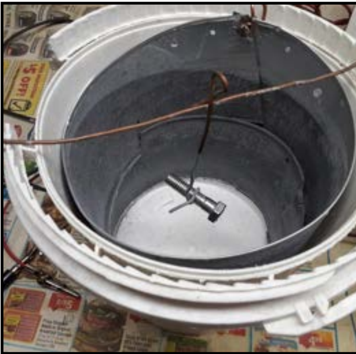
Here is a bolt set up for plating. There is no electrolyte in the bucket for photo purposes.
