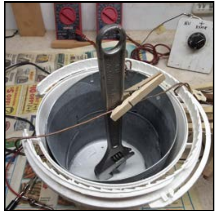
Here is a wrench being used to demonstrate that even parts too big to fully immerse can be plated. The clothes pin is holding the wrench to the hanger wire to complete the circuit.
